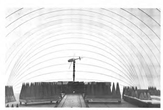
MURINE DETECTOR SYSTEM, developed by Division 2125 to protect Army helicopters from heat-seeking ground launched missiles, is on board this model helicopter. System is undergoing tests in the "bubble" antenna test range in Area III. Pointed shapes are microwave energy absorbing forms.
